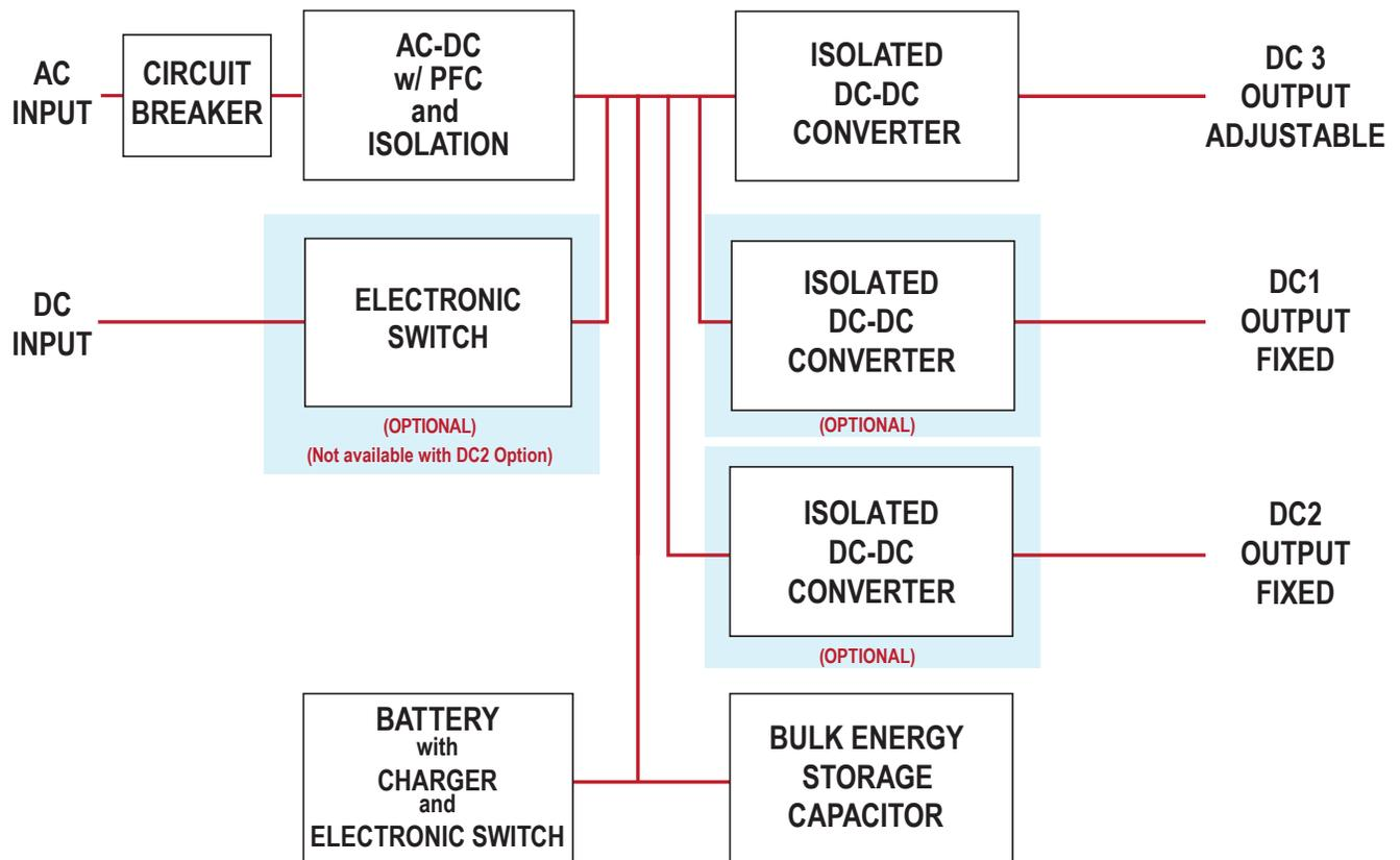
Power flows from the AC INPUT through an AC-DC converter that has Power Factor Correction (PFC) and high voltage safety isolation. Power flows from the DC INPUT through an electronic switch that is closed when the AC INPUT power is absent and the DC INPUT voltage is within its specified range. Otherwise, a second electronic switch is closed to connect the battery to the mid-bus.
