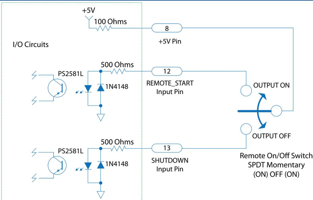
Note: A 2PDT or 3PDT switch may be substituted for single control of 2 or 3 UPS machines, respectively.
