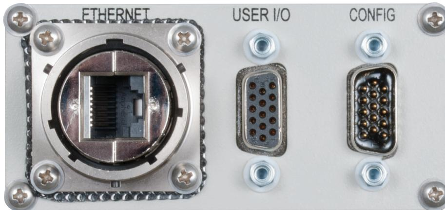
The User I/O female DB15 connector on the left is for a connection to a host/system computer so that it can control the UPS and receive information regarding the status of the UPS.
