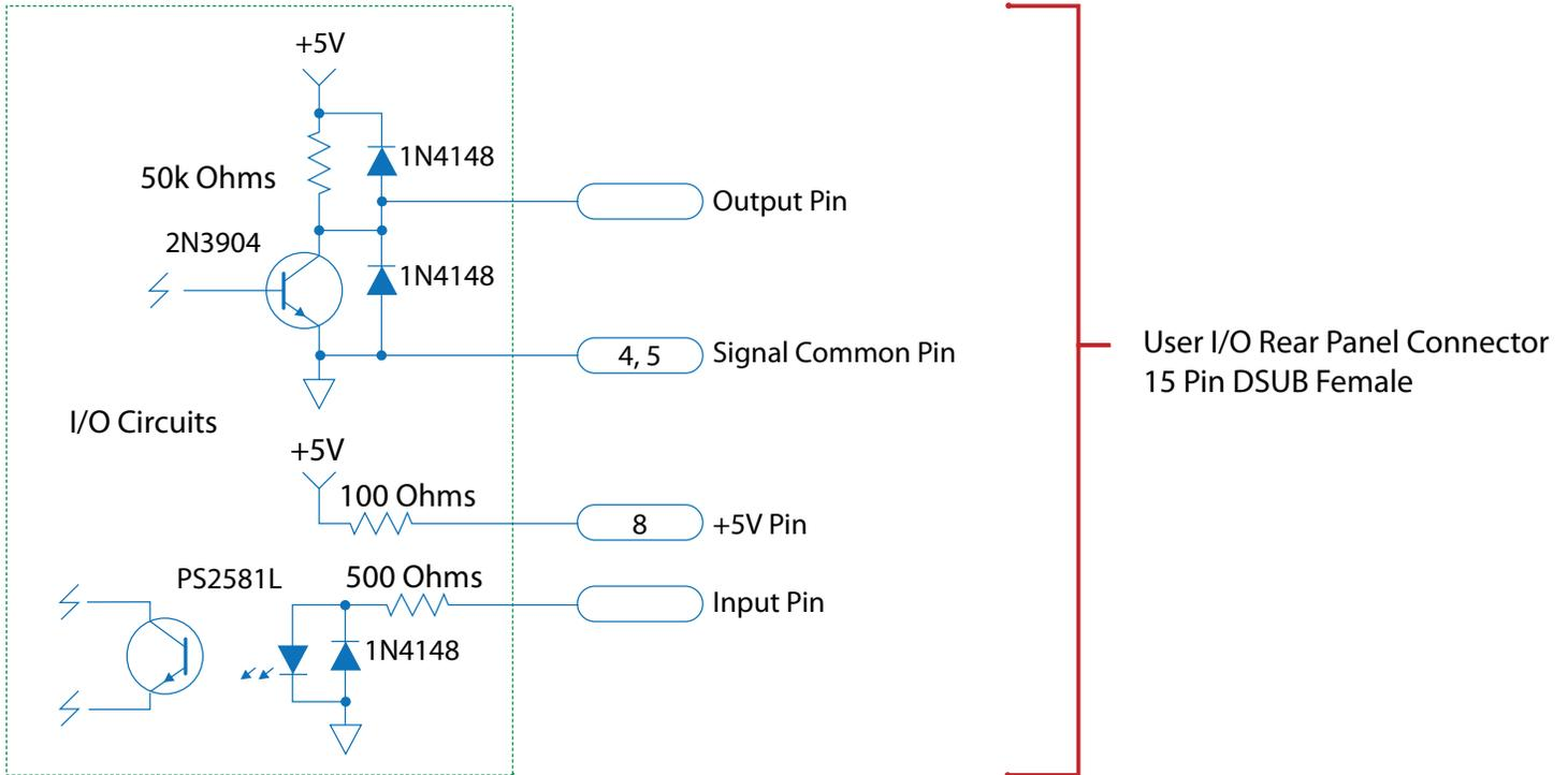
**Remote On/Off Switch Connections**
